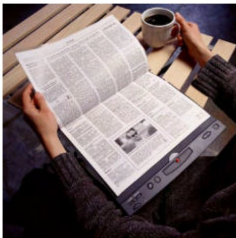
Concept e-newspaper from IBM – such concepts limited by a lack of affordable flexible substrates
