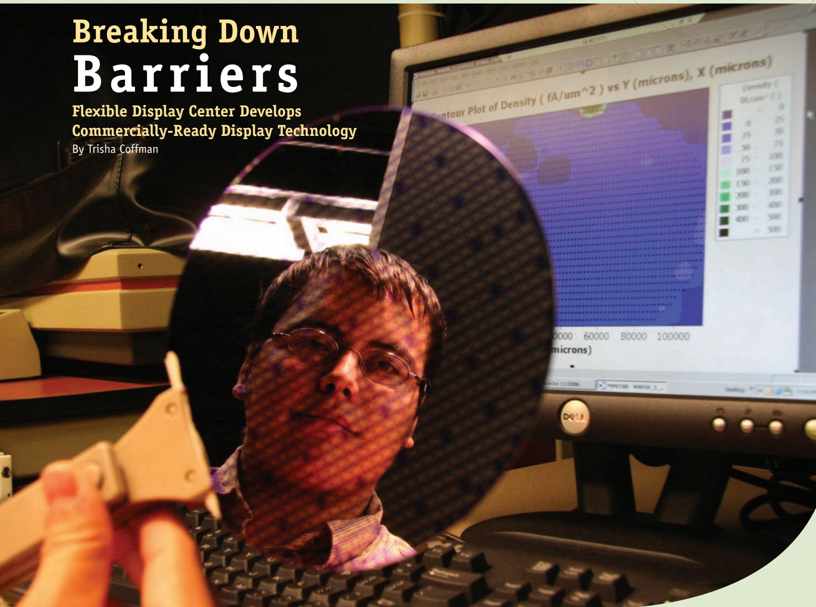
Graduate research assistant Jovan Trujillo shows a tantalum pentoxide film covered with more than 2,022 capacitor dots.
