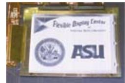
Engineers are striving to achieve flexible displays by using plastic and stainless-steel substrates, rather than glass.
